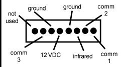
Each RJ45 connector uses 4 wires from MR60 to MVP64a for power, communications and IR. 3 are common, 12VDC, GND (either) and IR. 1 is uniqure 2-way comm (1, 2 or 3) Comm1 goes to keypad slot A1 or B1 Comm2 goes to keypad slot A2 or B2 Comm3 goes to keypad slot A3 or B3
